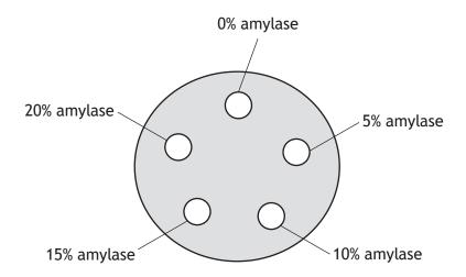
As the amylase diffuses out of the well it breaks down starch in the agar, turning the agar clear. The plates were incubated at 37 °C for 3 hours and the diameter of the clear zone around each well was measured using a ruler.
