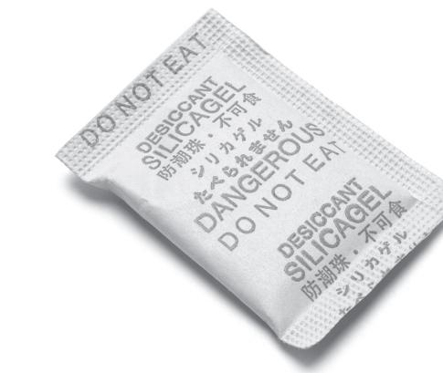
A small quantity of anhydrous cobalt(II) chloride,  $\text{CoCl}_2$ , may be added to the silica gel. A colour change from blue to pink is observed as the silica gel absorbs water. The pink colour indicates that the silica gel is no longer effective.
