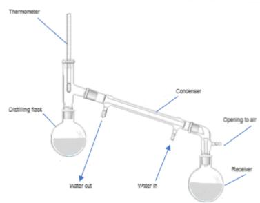
**IP6** inclusion of thermometer (pocket) on left-hand side (in this diagram) **and** opening for gaseous escape on right-hand side (in this diagram)
